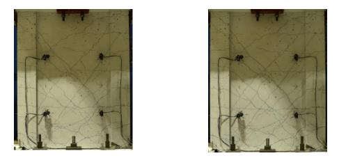
Figure 6. Crack pattern of the test specimen: Left: at the end of GM1; and Right: at the end of GM2.
