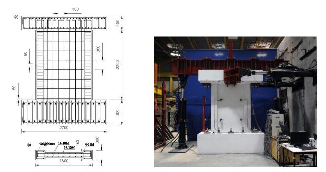
*Figure 2. Test specimen dimensions and test set-up: Left (a) elevation of the specimen; Left (b) cross section of the test specimen; and Right: test set-up.*
