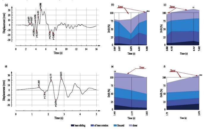
Figure 5. Displacement history of control point and displacement decomposition: (a) history under GM1; (b) decomposition in positive direction under GM1; (c) decomposition in negative direction under GM1; (d) history under GM2; (e) decomposition in positive direction under GM2; and (f) decomposition in negative direction under GM2.
