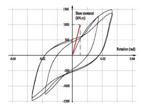
Figure 9. Extracting the rotation corresponding to development of the yielding moment at the wall base.
