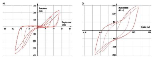
Figure 7. Pushover test results: a) base shear force demand; and b) flexural moment demand.
