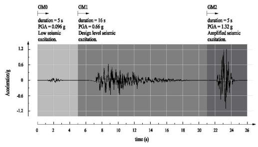
Figure 3. Applied seismic excitations.
