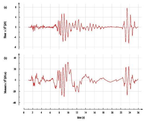
Figure 4. Seismic demands at the base of the reference RC wall: (a) shear force and (b) flexural moment.
