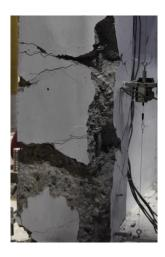
Figure 8. Bar buckling and loose broken concrete of the RC wall after the pushover test.
