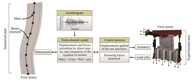
Figure 1. Hybrid test overall procedure and substructuring technic.
